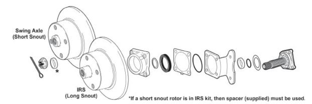
STEP 5: (See parts break down illustration) Install the bearing thrust washer, small o-ring, and original spacer on axle (Small o-ring not required on I.R.S.). Install the caliper bracket and large o-ring on the bearing flange. Install the bearing seal cap with new seal and oil deflector. Using only 1 gasket between bearing cap and caliper bracket. Torque the bearing seal cap bolts to 25 ft. lbs.
