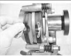
install the brake pads into caliper bracket against the rotor.
