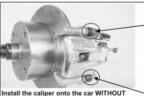
Install the caliper onto the car WITHOUT the brake pads. When installing make sure that the bleeder valve is in the up position on that specific side.
