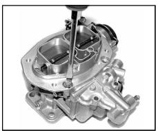
2. Remove the 5 mounting screws from the top of the carburetor and remove the top. Be careful not to tear the gasket.
