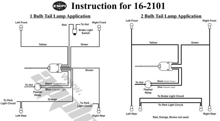
Consult relay manufacture's specifications for terminal identification. Connect the black wire to the switch or load terminal. Connect the blue wire to the pilot or dash lamp terminal. A flasher relay designed for a grounded dash lamp must be used or lamp in switch will continuously glow. Attach switch to steering column with clamp provided. Housing must be clamped to bare metal on column to ground switch assembly.
