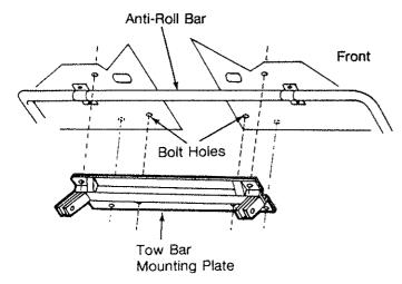
3. The holes on the flanges of the mounting plate line up with existing bolts on the underside of the car. All cars have two existing bolts in the front of the sway bar. Behind the sway bar there are usually four bolts, but sometimes only two will be found. (See diagram)
