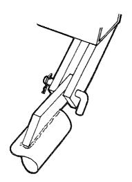
8. Adjust the coupler to correctly fit the ball as shown in the diagram below.
