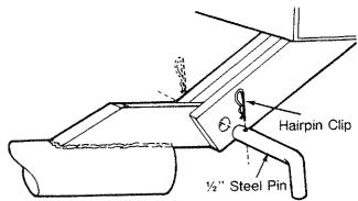
7. Snap the spring clips through the small holes in the end of the pins. It is vital to make sure that the clips are fully on the pins. They must be right up to the larger hole in the clip. (See diagram)
